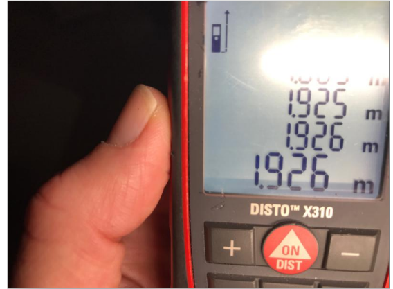
Photo - 75 Ridge height of pitched roof.
